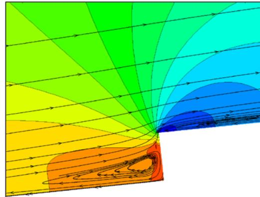
Pressure distribution and streamlines at a forward facing step
