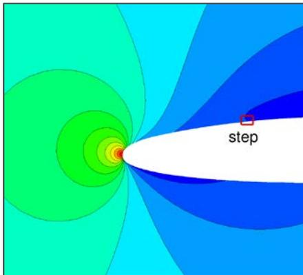
Pressure distribution on a laminar wing with step
