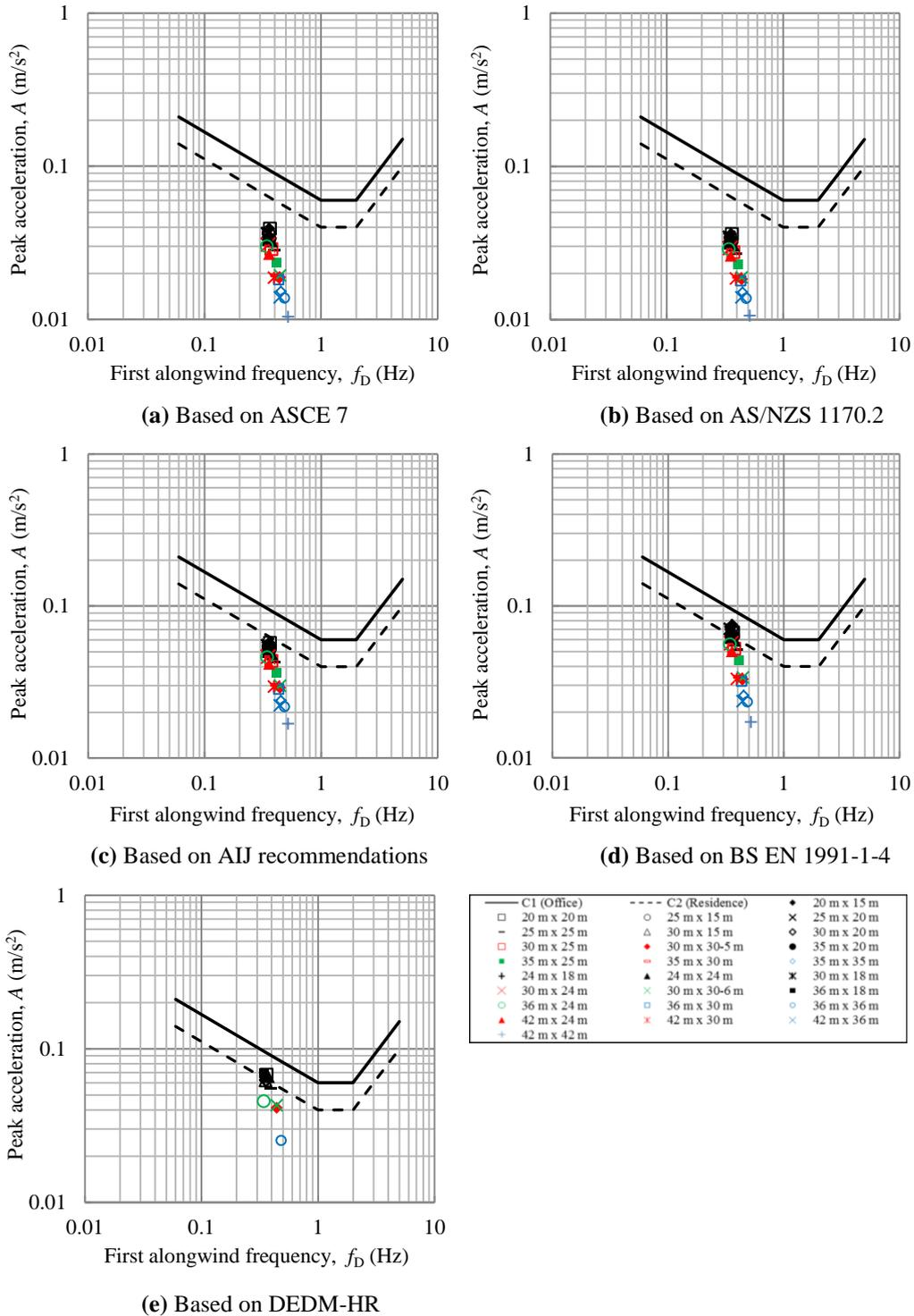
**Fig. 2** Evaluated alongwind peak acceleration responses to various design codes/standards and online design module for 40-storey buildings with  $\zeta = 0.01592$
