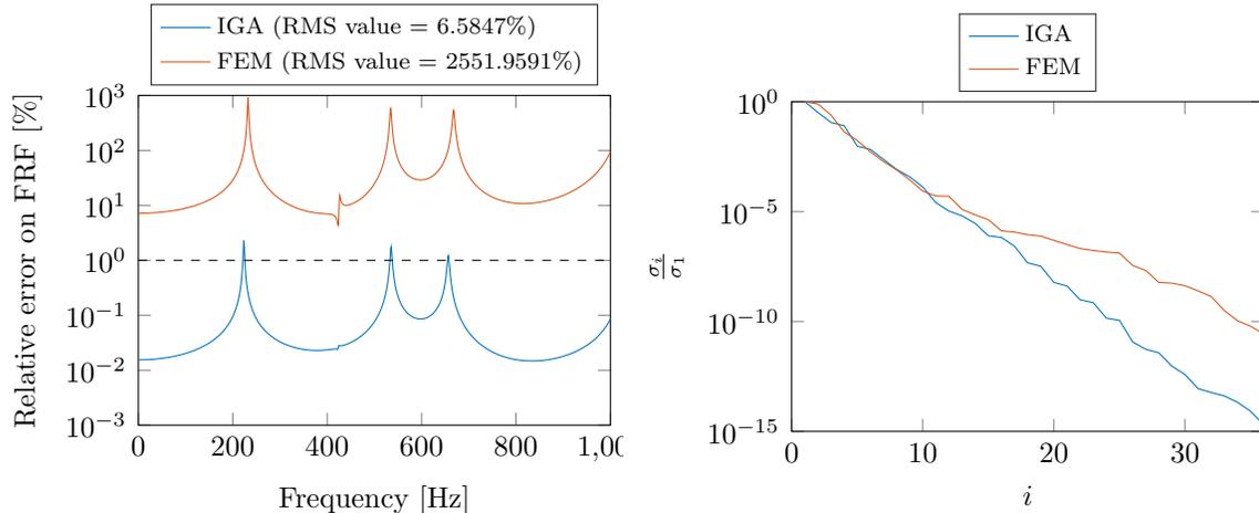
Figure 2: Reducibility for the curved beam. (Left) Reduction errors on the FRF (in %). (Right) Relative magnitude of the singular values.
