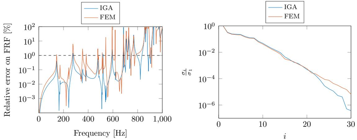
Figure 4: Reducibility for the acoustic cavity. (Left) Reduction errors on the FRF (in %). (Right) Relative magnitude of the singular values.
