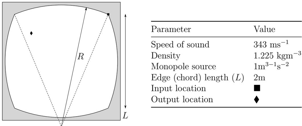
Figure 3: Problem definition of the acoustic cavity.
