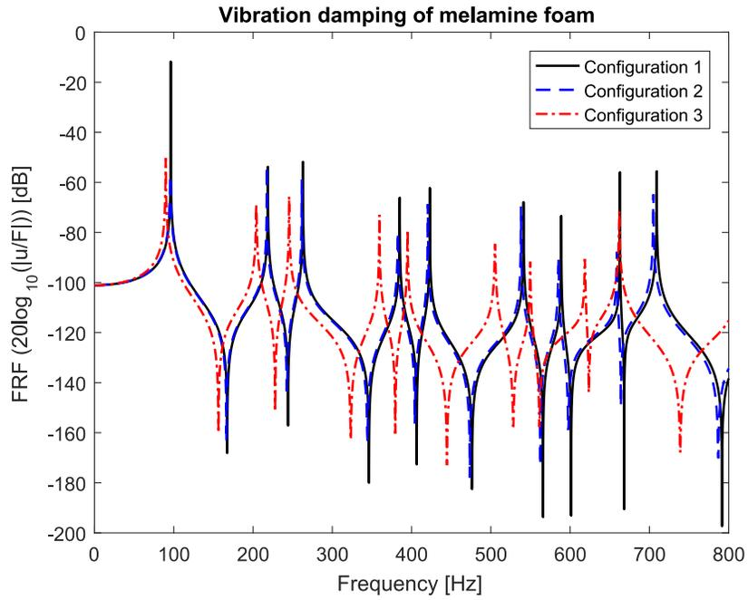
Figure 8: Frequency responses of the panel for configurations 1 to 3 using melamine foam.
