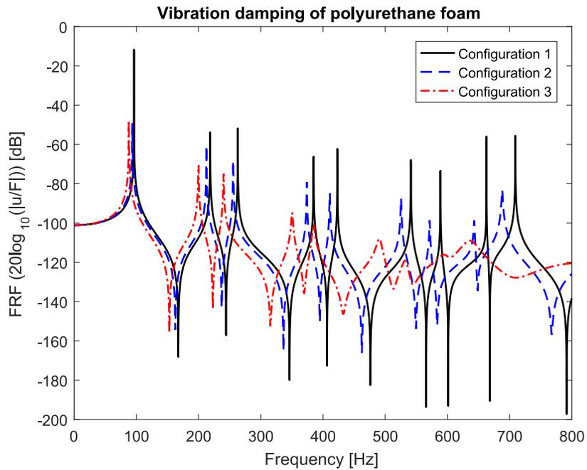
Figure 9: Frequency responses of the panel for configurations 1 to 3 using polyurethane foam.
