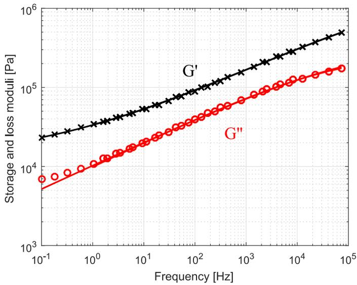
**Figure 5:** Dynamic shear modulus at 20° C for the polyurethane foam. Measurements (markers) and identified viscoelastic model (straight line).
