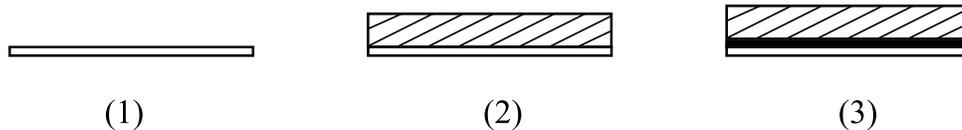
**Figure 6:** Three configurations under study. Aluminum panel (white), Rubber material (black), Poroacoustic material (hatched).
