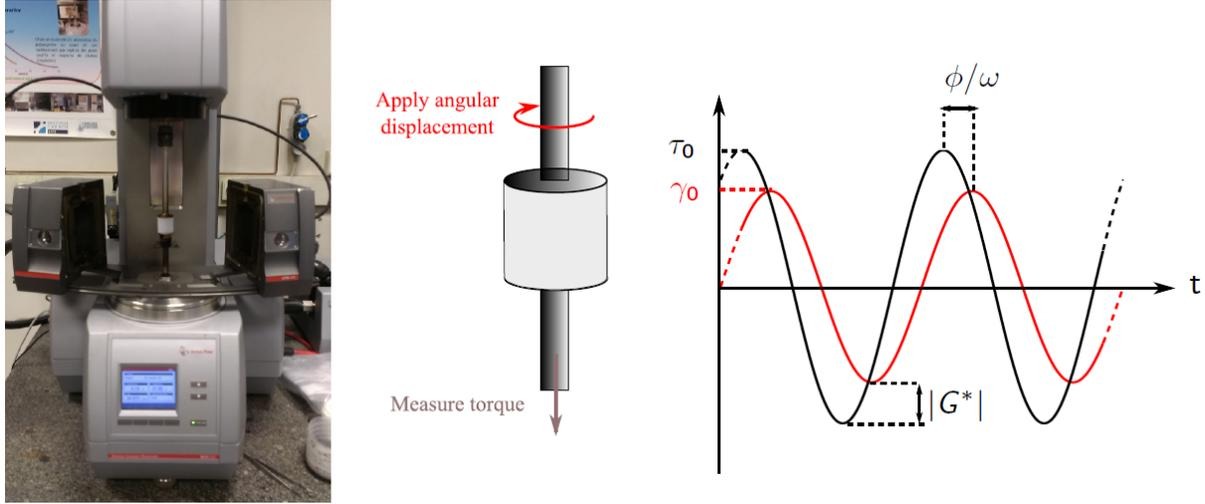
**Figure 1:** Oscillatory rheometer in torsion MCR 502 (Anton Paar).
