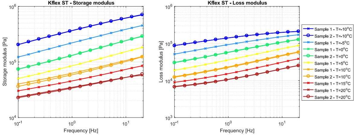
**Figure 3:** Storage and loss shear moduli for polyurethane foam samples.
