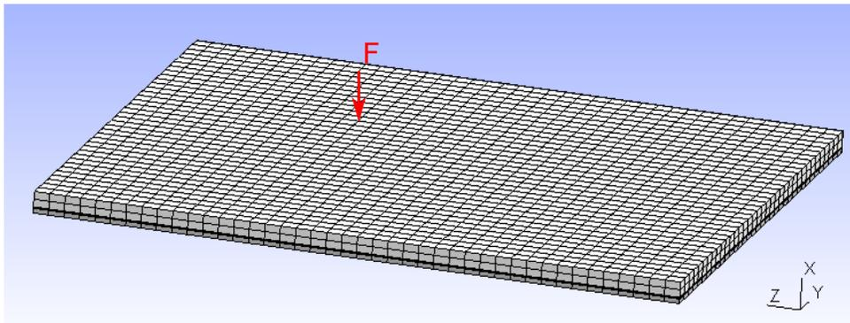
**Figure 7:** Finite element mesh for configuration 3 and location of the unit load point.
