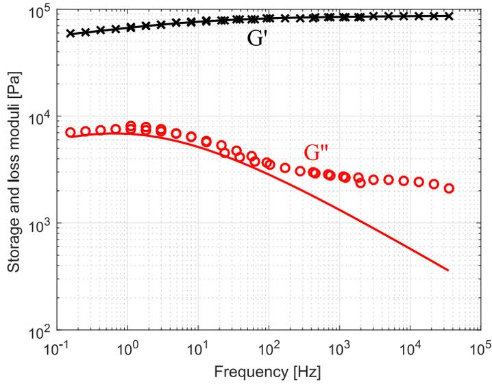
**Figure 4:** Dynamic shear modulus at 20° C for the melamine foam. Measurements (markers) and identified viscoelastic model (straight line).
