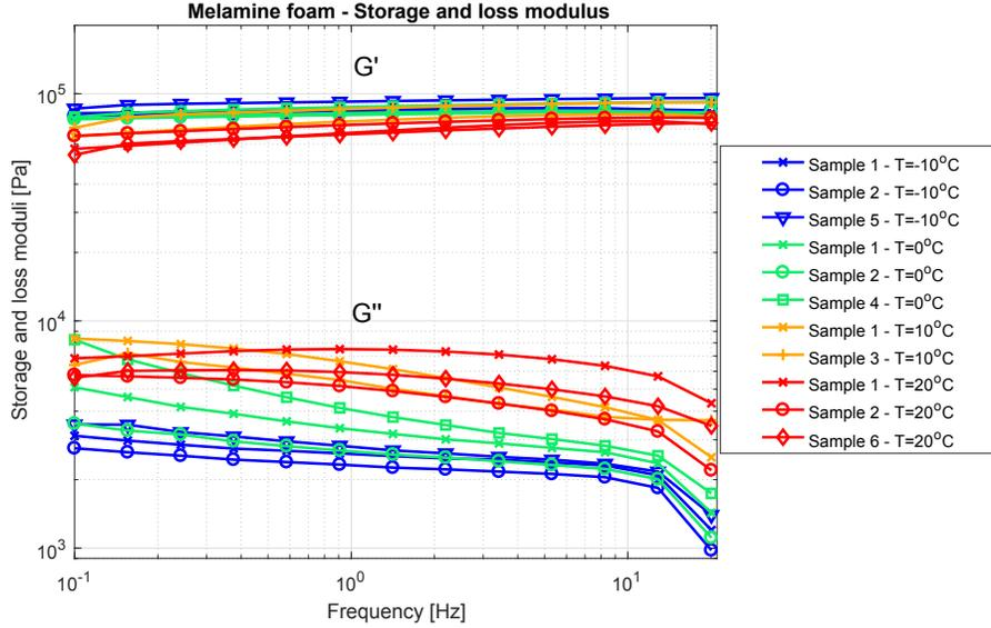
**Figure 2:** Storage and loss shear moduli for melamine foam samples.
