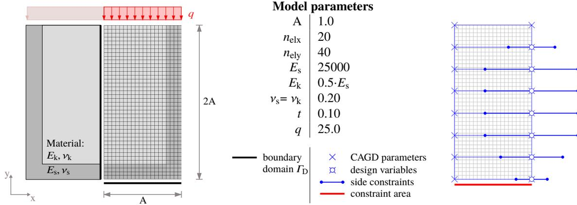
**Figure 1:** Domain with multi-material: mechanical system, FE-mesh, boundary conditions and load case, model parameters and optimisation model (design variables, side constraints and constraints area)
