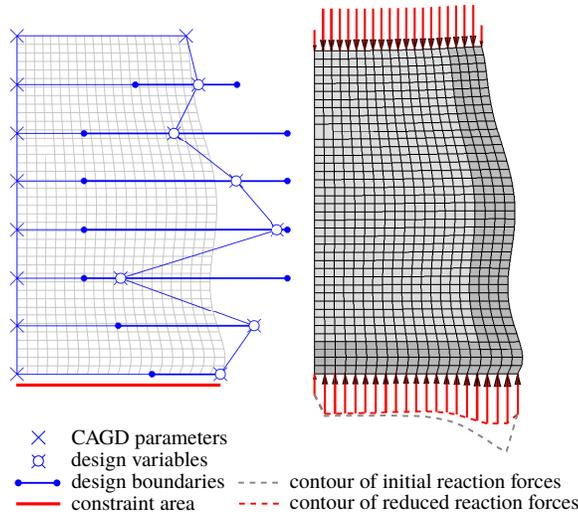
Figure 3: Optimal design and comparison of reaction forces for the deformed system (scaling( $v$ ) = 1.0)
