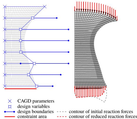
**Figure 5:** Optimal design and comparison of reaction forces for the deformed system (scaling( $\nu$ ) = 1.0)
