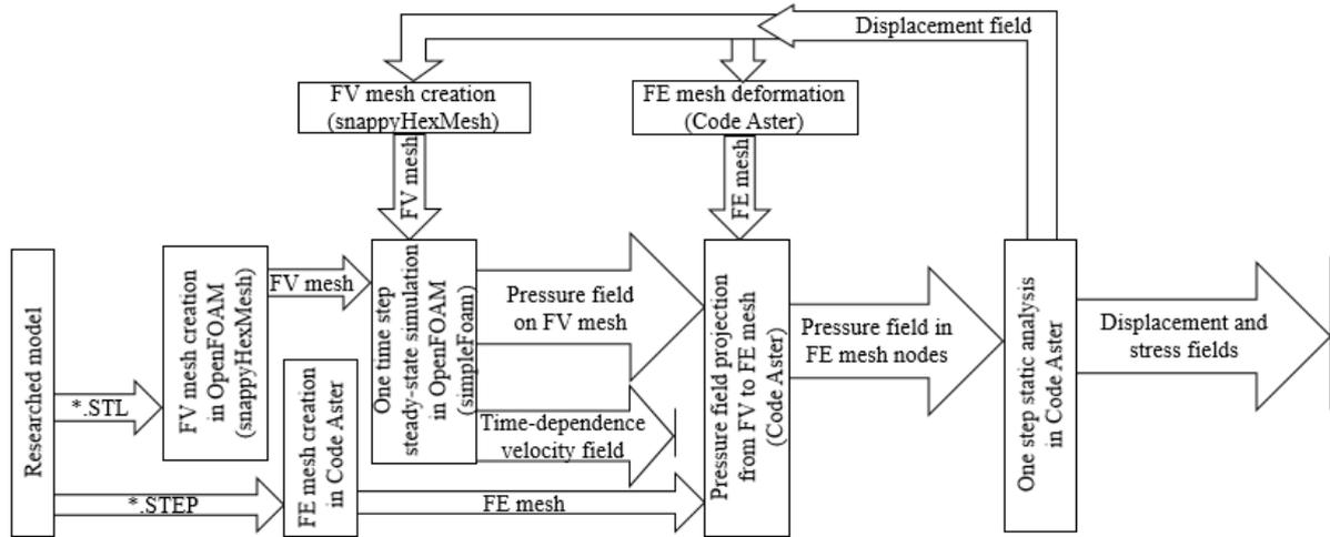
Figure 3: Simulation algorithm at quasistatic problem definition taking into account body
