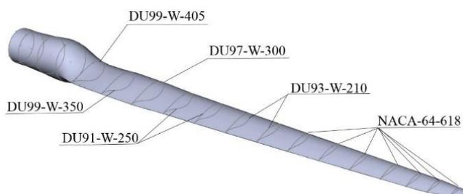
**Figure 5:** Researched blade of the wind turbine
