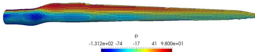
**Figure 8:** Aerodynamic pressure in the FV at the blade surface
