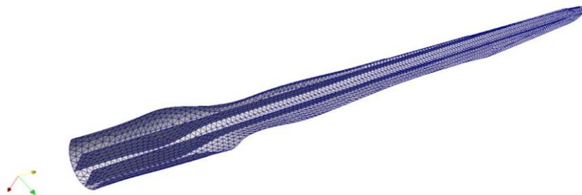
**Figure 9:** Finite element mesh of the blade (longitudinal section)
