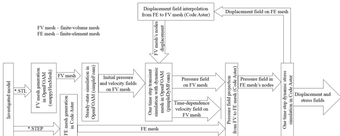
Figure 4: Simulation algorithm at two-way weak coupling problem definition
