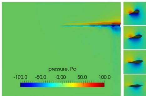
**Figure 6:** Pressure field at steady-state solution
