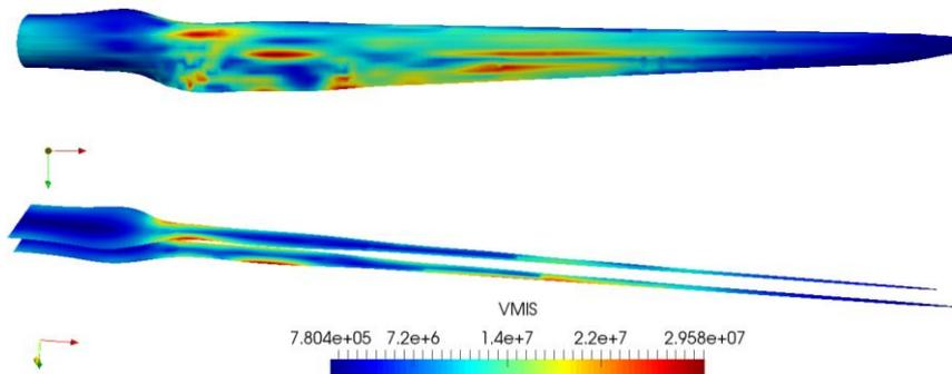
**Figure 12:** Plot of the stress (Von Mises): top - shell, bottom - longeron
