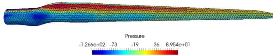
**Figure 10:** Pressure field interpolated to the FE mesh
