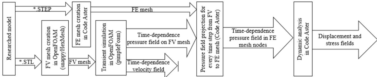
Figure 2: Simulation algorithm at dynamic problem definition
