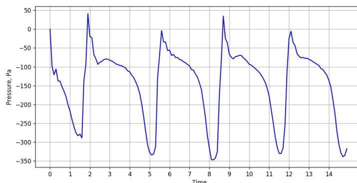
**Figure 16:** Pressure plots for point A near the surface of the blade
