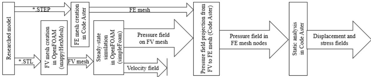
**Figure 1:** Simulation algorithm at quasistatic problem definition
