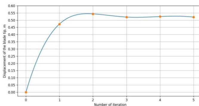
Figure 15: Displacement of the tip of the blade
