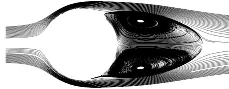
Figure 9: Streamlines along the separation region at a mid-plane slice of the sphere,  $\mathbb{P}^2$  approximation, embedded approach.
