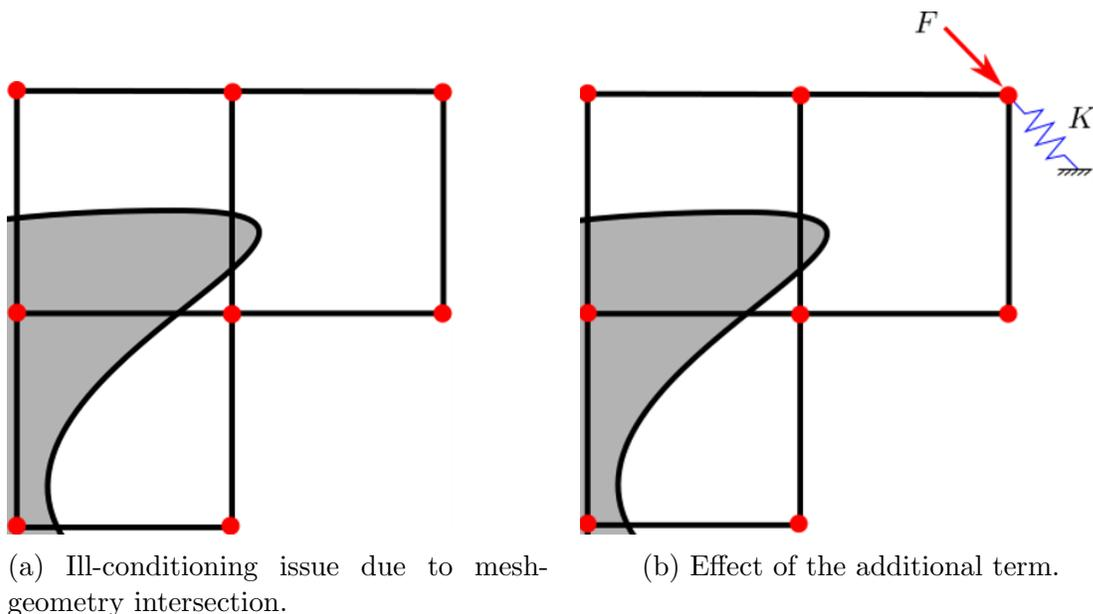
Figure 1: Scheme of an element subject to ill-conditioning issues. The stiffness of the nodes far from the domain (in grey) is small.
