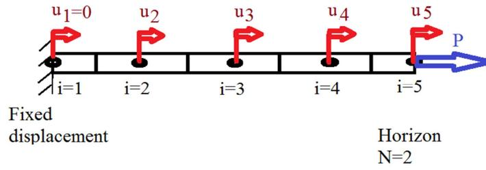
**Figure 5:** A peridynamic model of an SMA rod used in simulations of the superelasticity effect.
