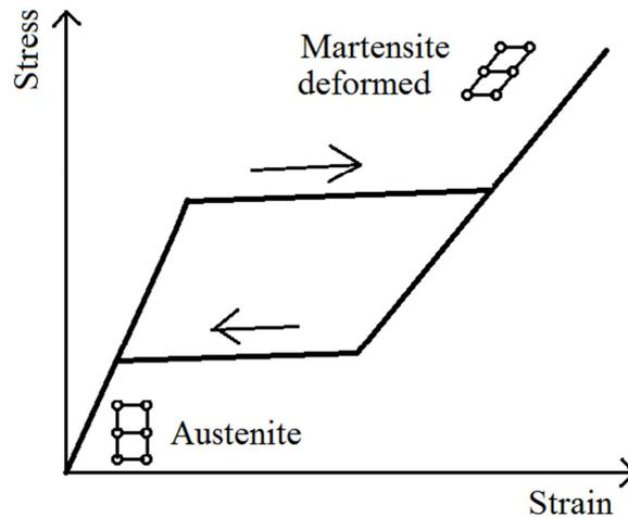
**Figure 4:** Stress-strain path for superelasticity – full cycle of mechanical loading and unloading an SMA sample.
