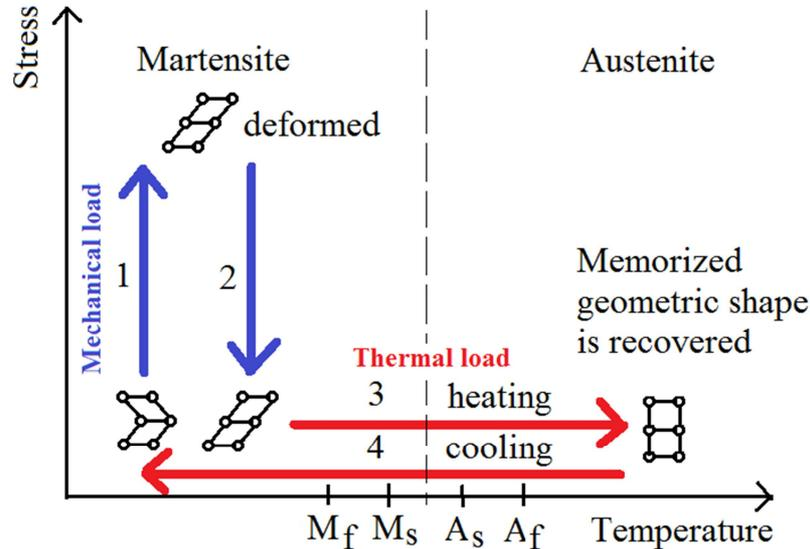
**Figure 2:** One-way memory effect – application of thermal load is used to recover remembered shape
