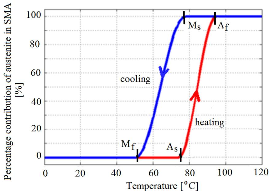
**Figure 1:** Austenite contribution during reversible phase transition processes activated by the temperature change
