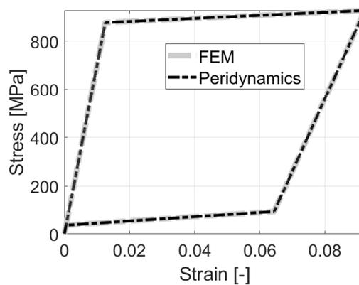
**Figure 6:** Stress-strain paths observed for the superelasticity effect.
