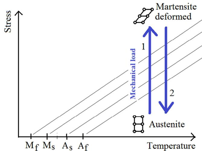
**Figure 3:** Reversible behavior of SMA for superelasticity – full cycle deals with mechanical loading and unloading an SMA sample.
