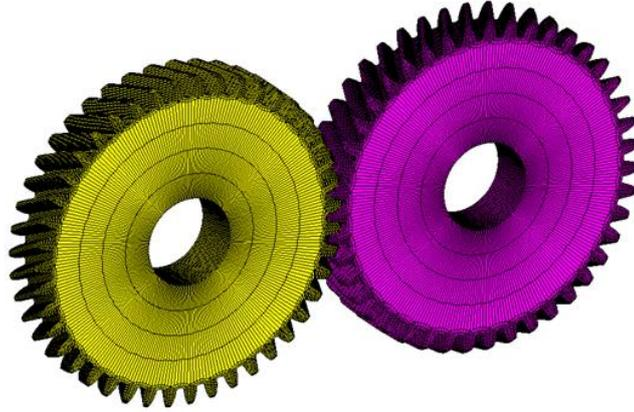
Figure 1. Helical gears for gear profile modification
