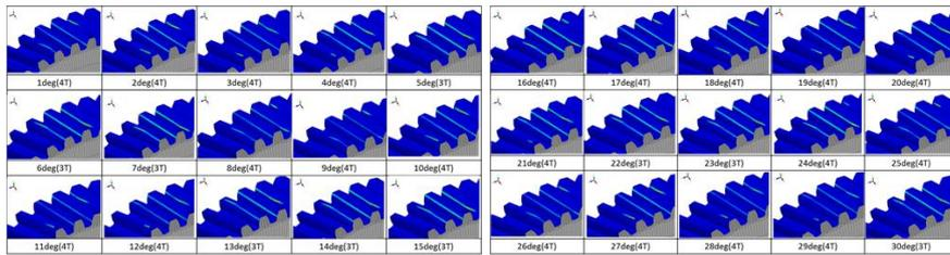
(b) Teeth contact pattern according to a rotation angle
