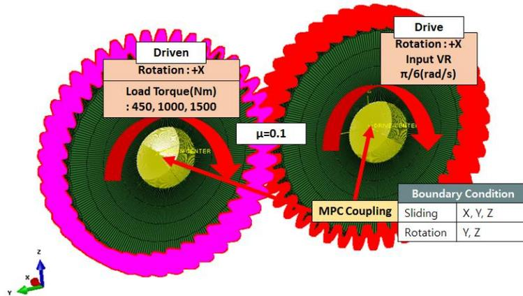
Figure 2. Boundary condition for gear profile modification
