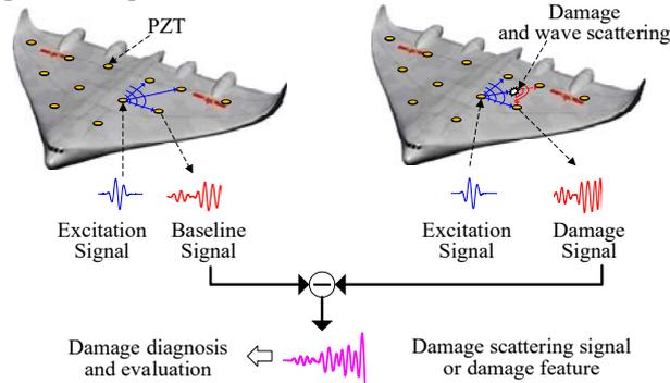
Figure 2: Illustration of the active guided wave based SHM
