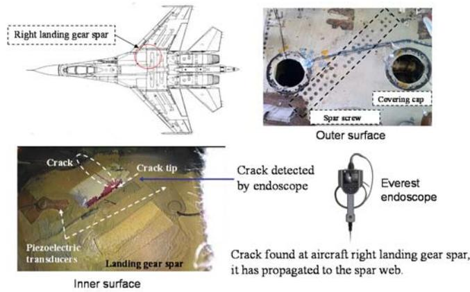
**Figure 3:** Experimental setup of the full-scale fatigue test
