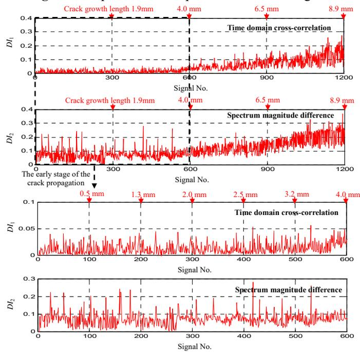
**Figure 4:** Signal features extracted from guided wave signal
