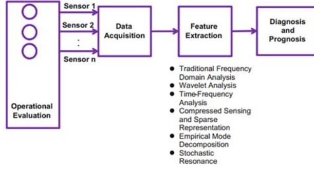
Figure 1: Typical process of SHM [9]
