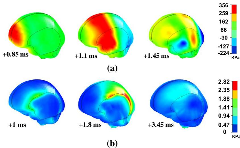
**Figure 3:** Variation of (a) ICP and (b) shear stress in the brain tissue for the Inclusive model
