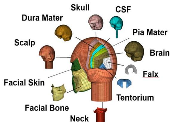
**Figure 1:** Finite Element model of the head
