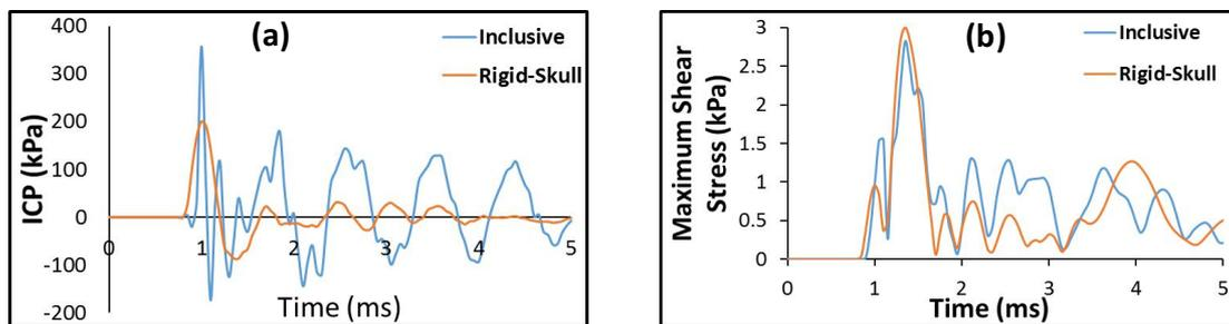
**Figure 4:** Comparison of time history of (c) ICP and (d) shear stress in the regions of maximum pressure and shear stress between inclusive and rigid-skull models
