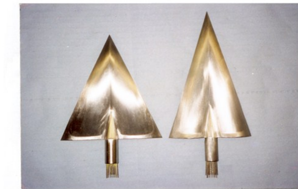
Figures 2a,b: The views of GO shapes of fully- integrated wing-fuselage models Fadet I and Fadet II
