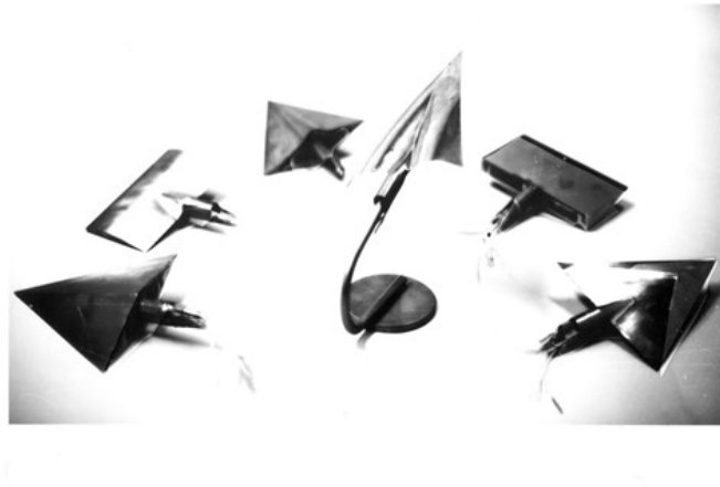
Figures. 1 The global optimized delta wing model Adela and others five non optimized FC models
