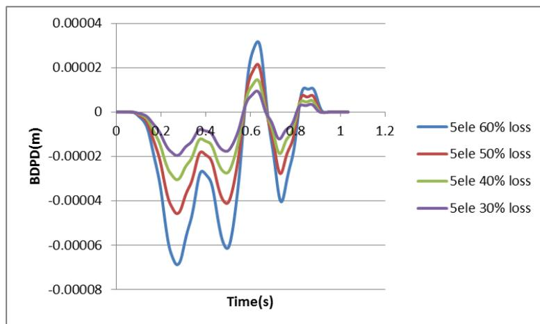
**Figure 5:** BDPD for different damage levels in Element 5
