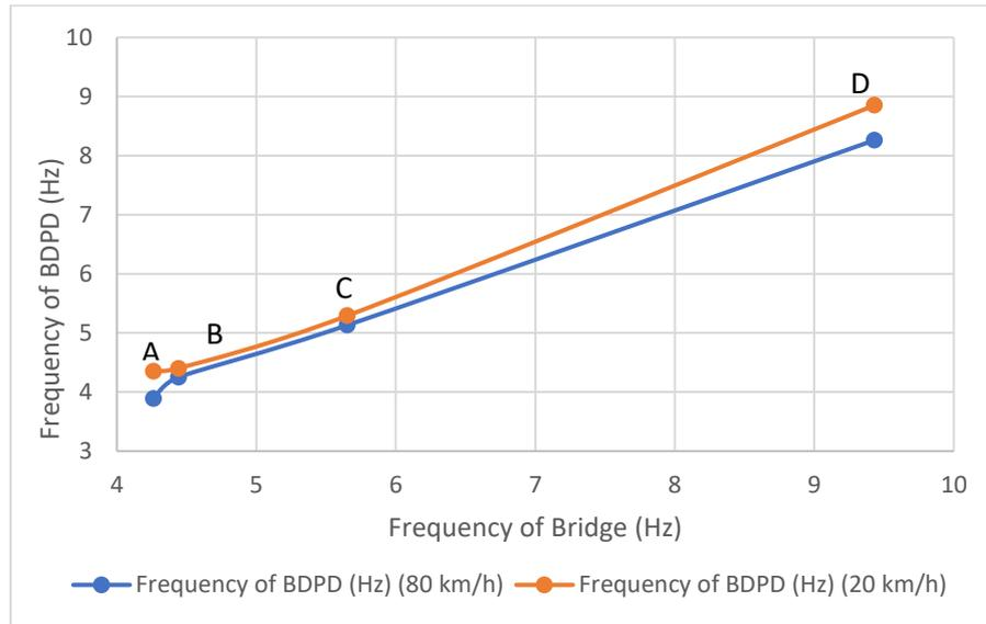
**Figure 4:** The relationship between the frequency of BDPD and the frequency of the bridge
