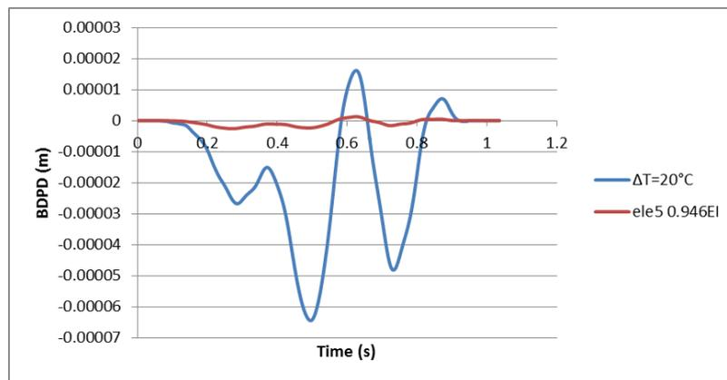
**Figure 7:** The BDPD because of damage effect and temperature change effect
