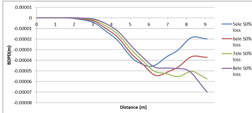
**Figure 6:** The BDPD for different damage locations (Element 5, 6, 7 and 8 of 20)
