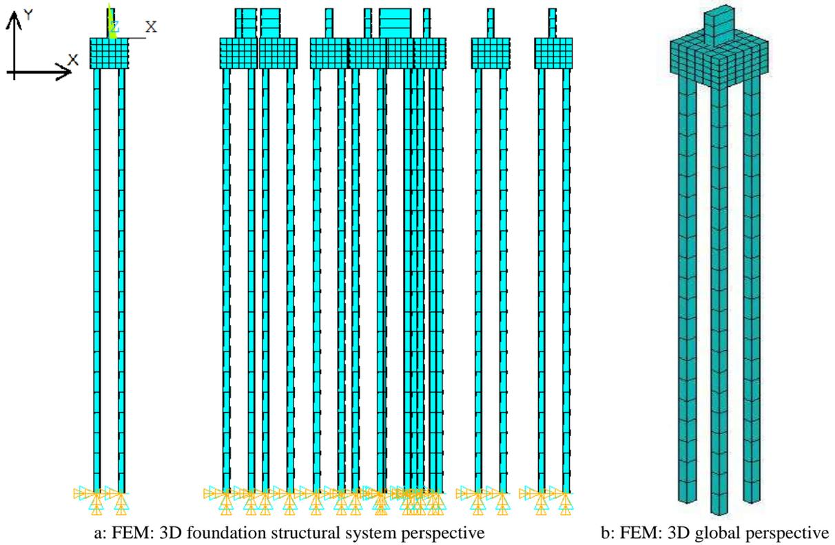
**Figure 6:** Views of the foundation's numerical model
