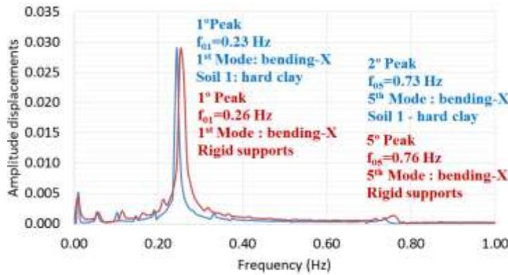
**Figure 15:** Accelerations at the top of the building in the frequency domain
