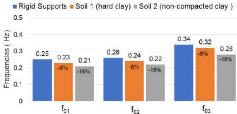
Figure 9: Comparison between frequencies - (1<sup>st</sup> to 3<sup>rd</sup> modes)
