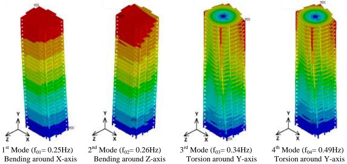
**Figure 7:** Building vibration modes with rigid supports
