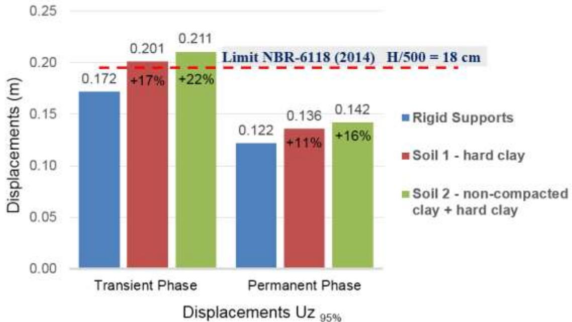
**Figure 12:** Investigated building nondeterministic structural response: maximum displacements
