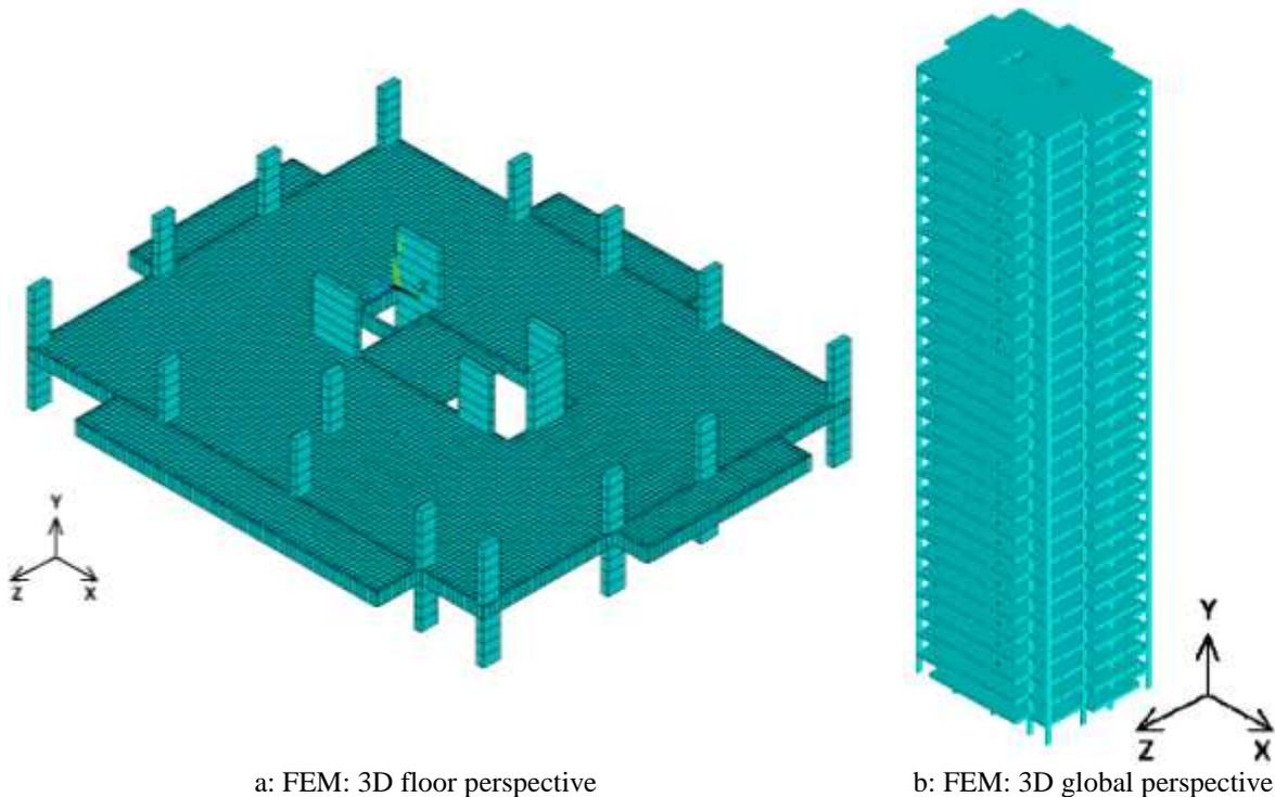
**Figure 5:** Finite element model of the investigated 30 story building [1]
