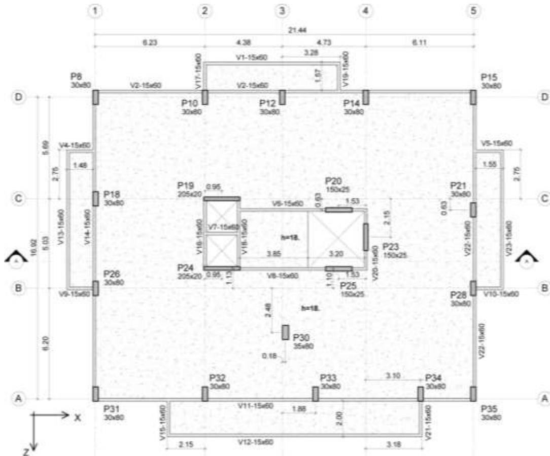
Figure 1: Investigated building: floor structural plan (units in meters)
