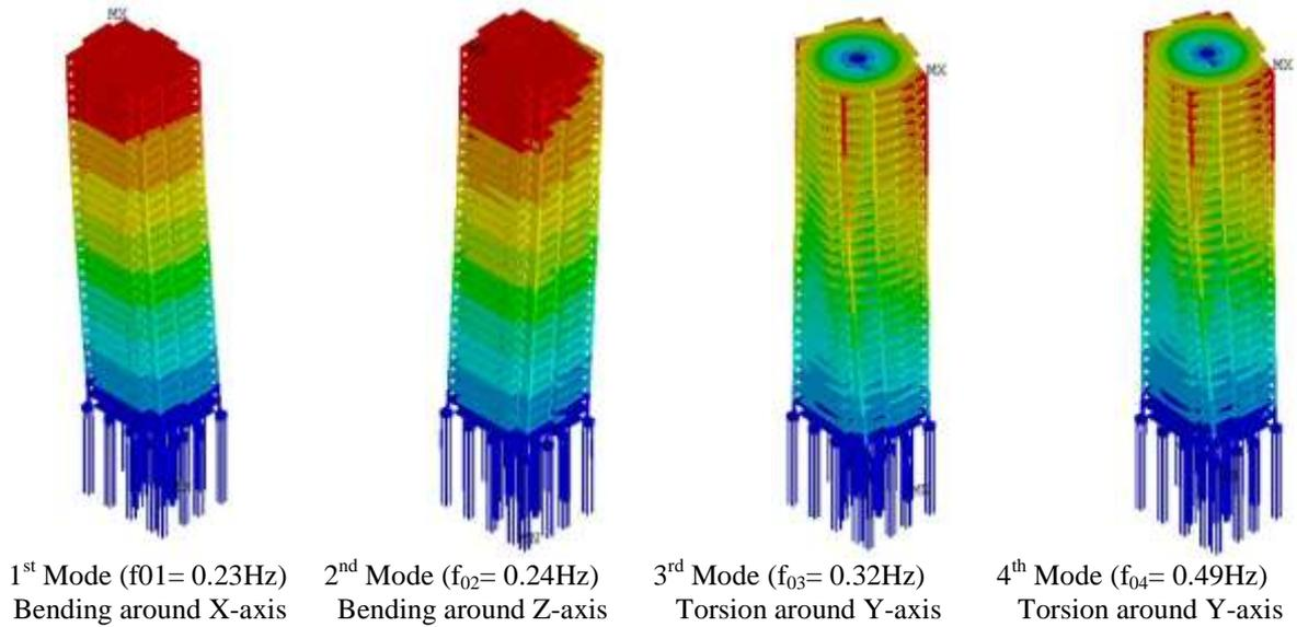
**Figure 8:** Building vibration modes with soil-interaction (Soil 1: hard clay)
