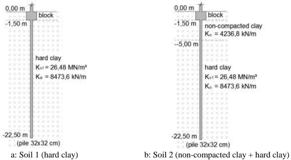
**Figure 3:** Geotechnical profile of the investigated soils
