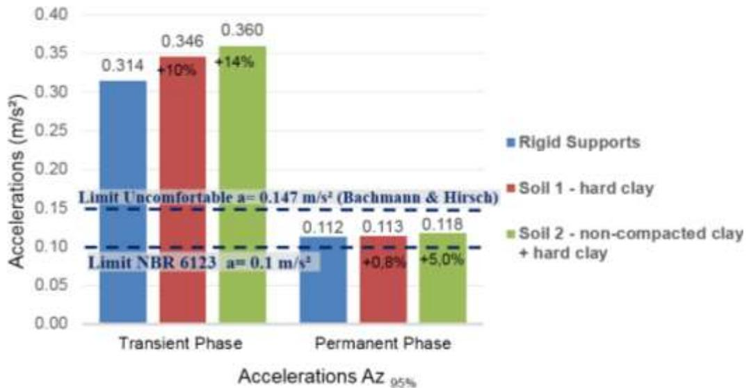
**Figure 14:** Investigated building nondeterministic structural response: maximum accelerations
