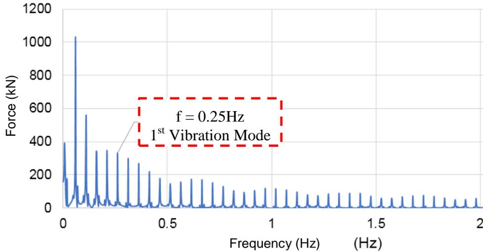
**Figure 11:** Nondeterministic wind action in frequency domain
