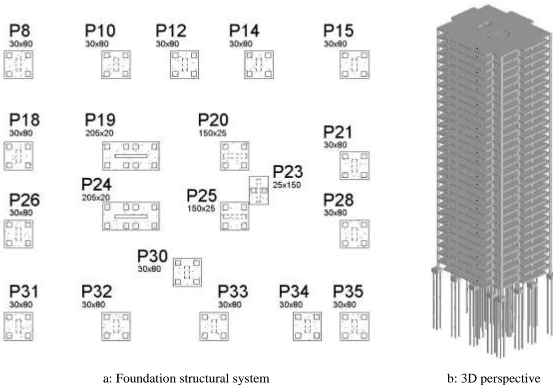
**Figure 4:** Structural model of the investigated foundation system
