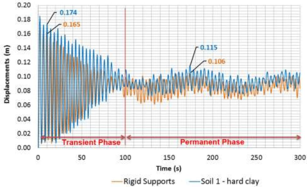
**Figure 13:** Horizontal translational displacement at the top of the building in the time domain
