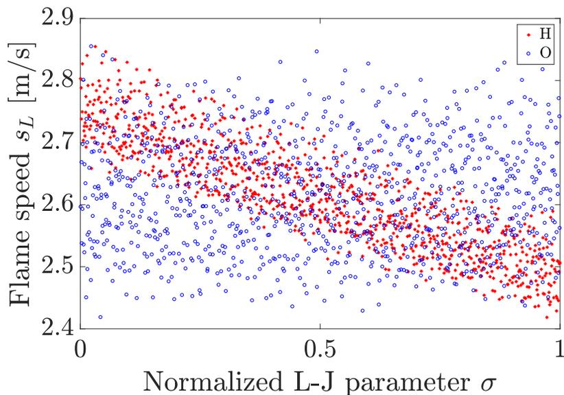
Figure 3: Flame speed  $s_L$  vs. the collision diameter  $\sigma$  of H, O.
