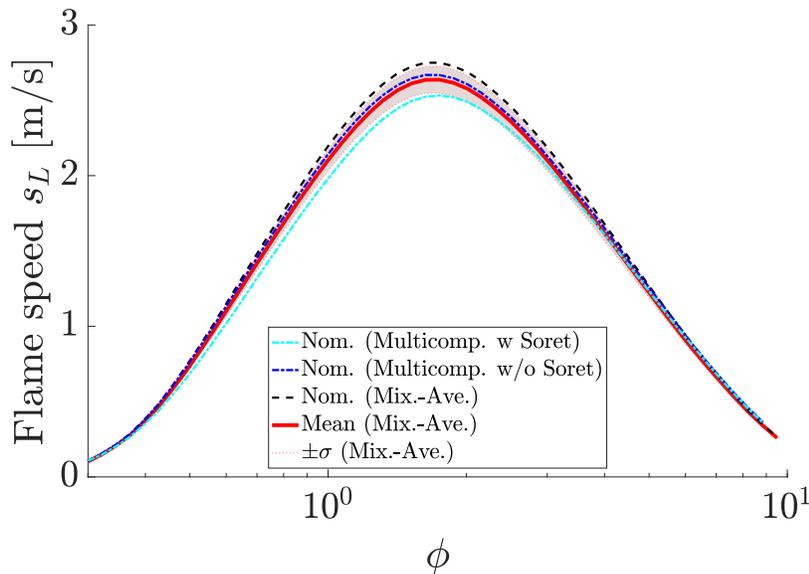
Figure 1: The variation of flame speed  $s_L$  with respect to the equivalence ratio  $\phi$ , and the uncertainty of  $s_L$  due to transport properties.
