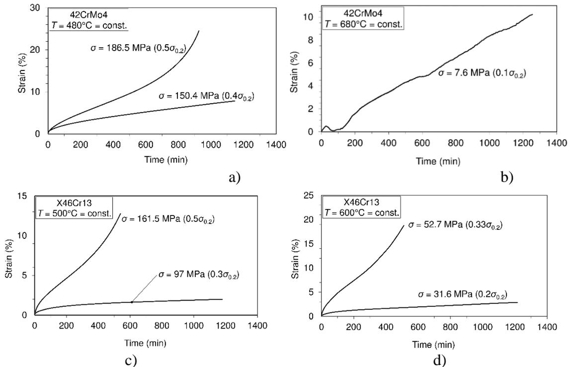
**Figure 3:** Short-time creep tests. a) Steel 42CrMo4 at temperature of  $480^\circ\text{C}$ . b) Steel 42CrMo4 at temperature of  $680^\circ\text{C}$ . c) Steel X46Cr13 at temperature of  $500^\circ\text{C}$ . d) Steel X46Cr13 at temperature of  $600^\circ\text{C}$
