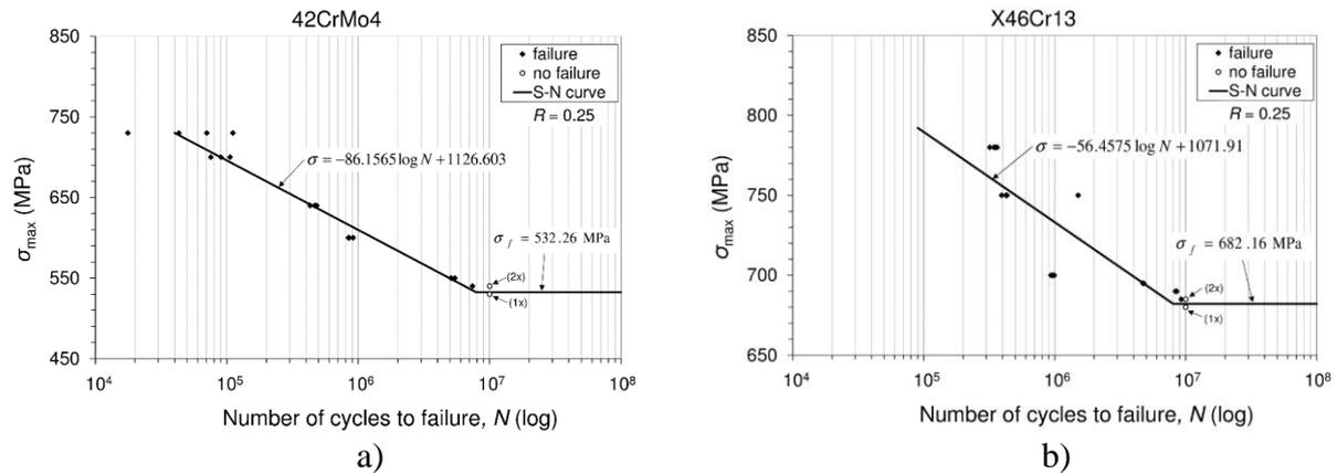
Figure 4: Fatigue tests and fatigue limit calculation. a) 42CrMo4 steel. b) X46Cr13 steel.
