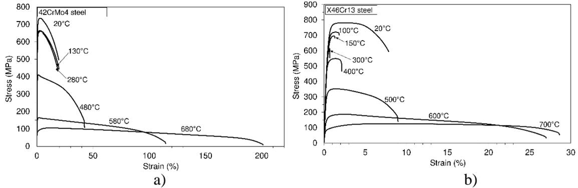
**Figure 2:** Engineering stress-strain diagrams. a) Steel 42CrMo4. b) Steel X46Cr13.
