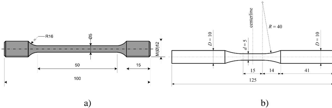
**Figure 1:** Geometry of the specimen used in these investigations. a) Uniaxial testing. b) Fatigue testing.
