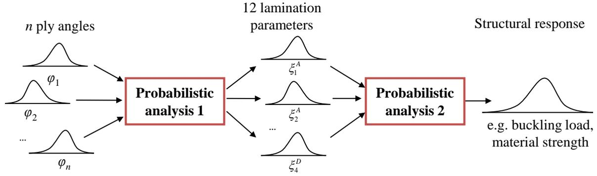
**Figure 2:** Two-step probabilistic analysis with ply angles as random parameters, using lamination parameters
