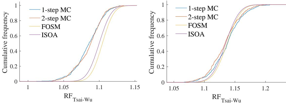
**Figure 3:** Cumulative distribution function of the reserve factor for the analytic example with load case A (left) and load case B (right)
