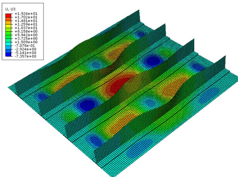
**Figure 4:** Postbuckling pattern of the considered stiffened composite panel
