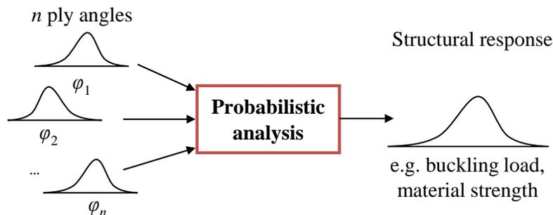
**Figure 1:** Probabilistic analysis with ply angles as random parameters
