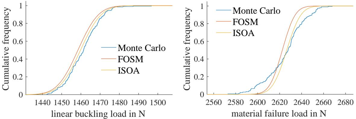
**Figure 6:** Cumulative distribution function of the linear buckling load (left) and material failure (right) of the stiffened panel for different approaches
