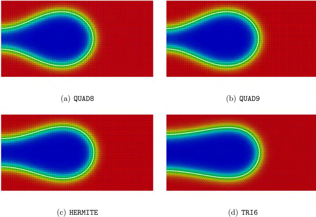
**Figure 3:** Equilibrium shape of Bi-concave example with different element types.
