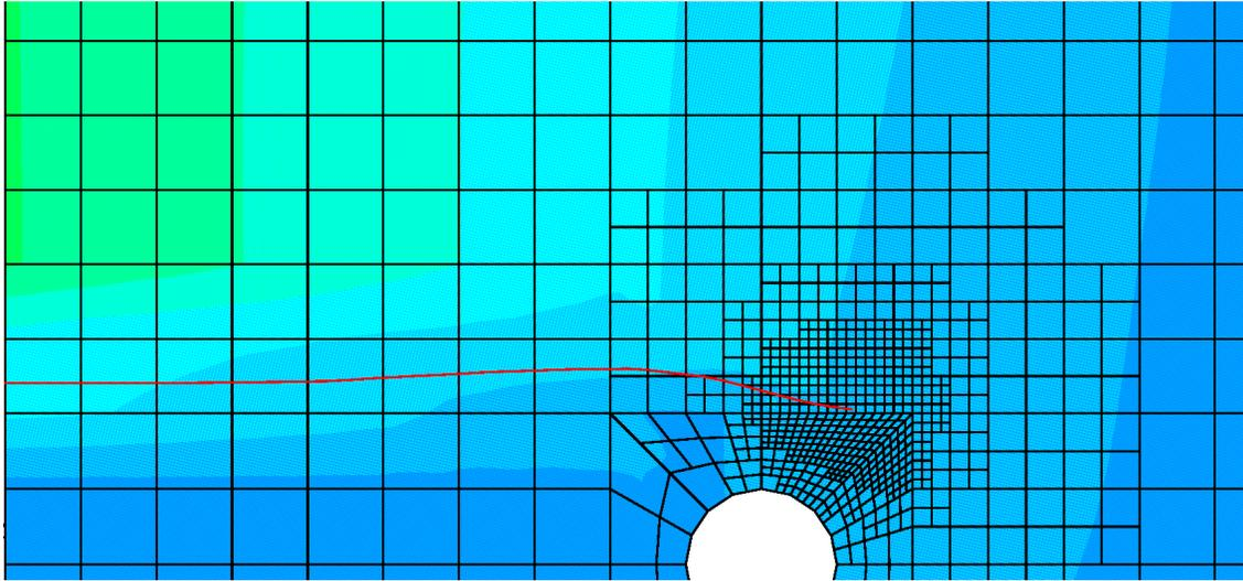
**Figure 1:** 2D mixed mode crack propagation
