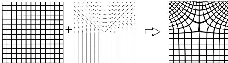
**Figure 1:** A regular grid (left) is distorted (right) according to a direction field featuring a singularity (center)
