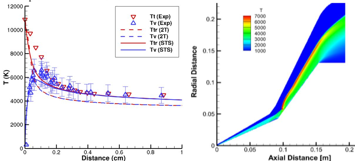
Figure 1: Assessment of high fidelity computation of: (a) Mach 12 shock wave; (b) Mach 12 flow over a double cone.
