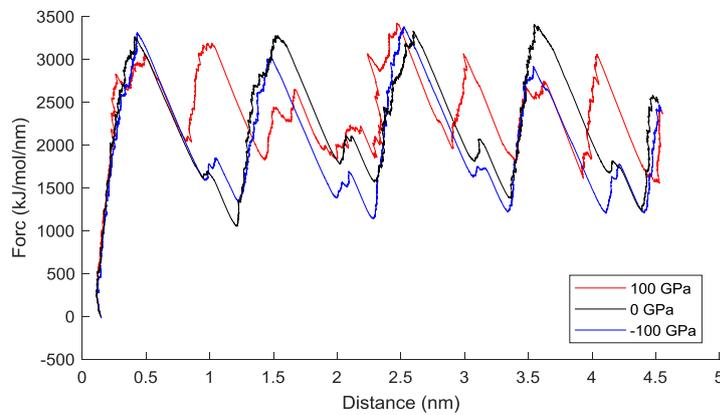
Figure 2 influence of compressional and tensile stresses on stick-slip behavior of dry interface between (110) and (110) plane, with main axes aligned, showing similar peak forces of the three conditions.
