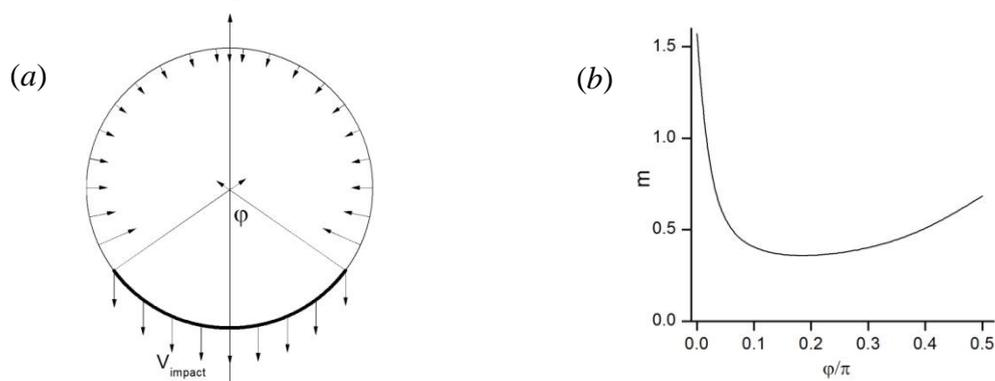
(a) Velocity along the cylindrical cavity generated by the impulsive motion of the circular arc, and (b) the added mass coefficient vs. the angle of the circular arc.
