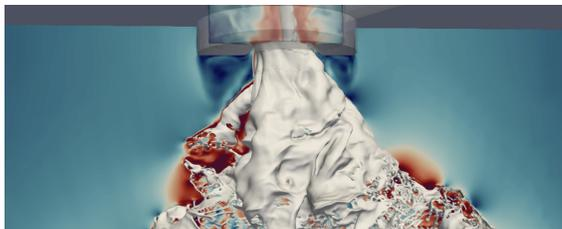
**Figure 1:** A hollow cone type spray is formed in the nozzle near field.
