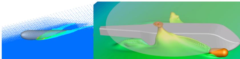
**Figure 1:** SPH simulation of airplane and helicopter ditching
