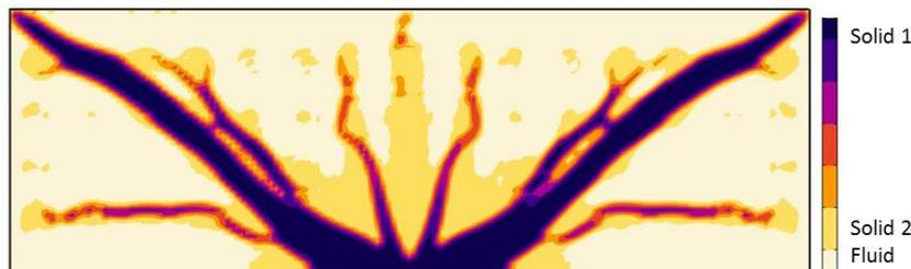
Figure 1 Optimised two-material convectively cooled heat sink design
