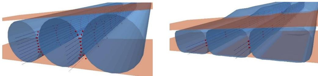
*beams before (left) and after (right) transversal compression, ribbon of contact (blue) and pairs of contact particles (red)*
