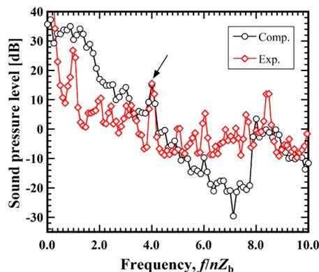
**Figure 1** Predicted and measured sound pressure spectra in upstream of fan.
