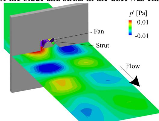
**Figure 2** Predicted contours of sound pressure fluctuations.
