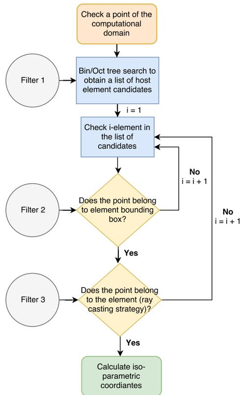
**Figure 1:** Flowchart of the point-location process.
