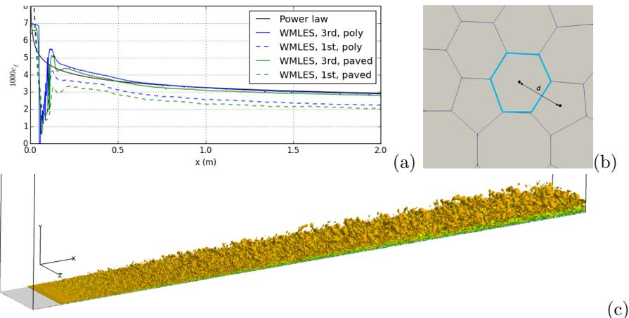
**Figure 1:** (a): Prediction of the friction coefficient along the plate. Comparison of different WMLES with a power law. (b) Illustration of the surface mesh for the polyhedral grid. The different grids are constructed so that the average distance between cell-centres,  $d$ , is the same. (c) The flow illustrated by an iso-surface of the second invariant of the velocity gradient, colored by axial flow velocity.
